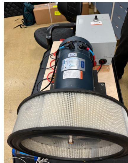
Figure 17: Packair Compressor Connected to a Motor and Air Filter.
